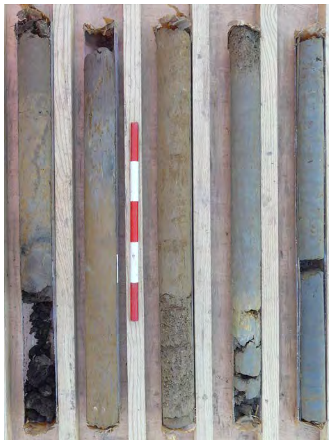
Plate 13: Weathered bedrock overlain by gravelly Head, sealed by brickearth and intercalated Holocene alluvial and peat deposits, Borehole OCA-WS304, 0-5m, Transect 3 (ground surface, top left)
