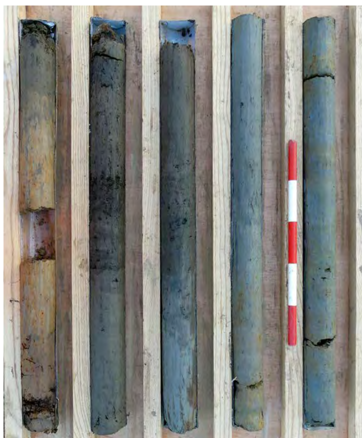
Plate 18: Organic and gleyed palaeochannel deposits (later prehistoric) overlying weathered bedrock, OCA-WS405A, 0-5m, Transect 4 (ground surface, top left)
