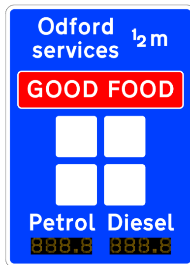
Figure 4.8 – Authorised non-prescribed sign with four placeholders and LED fuel prices
