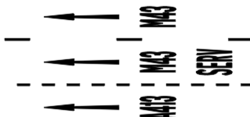
Figure 4.23 – Road markings on the approach to an MSA at a ghost island with lane drop and taper diverge junction
