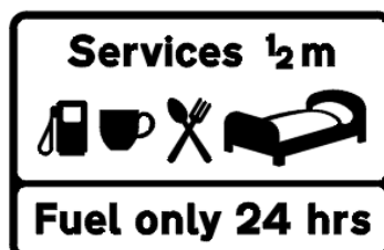
Figure 5.3 - Services 1/2 mile sign with only fuel available 24 hours
