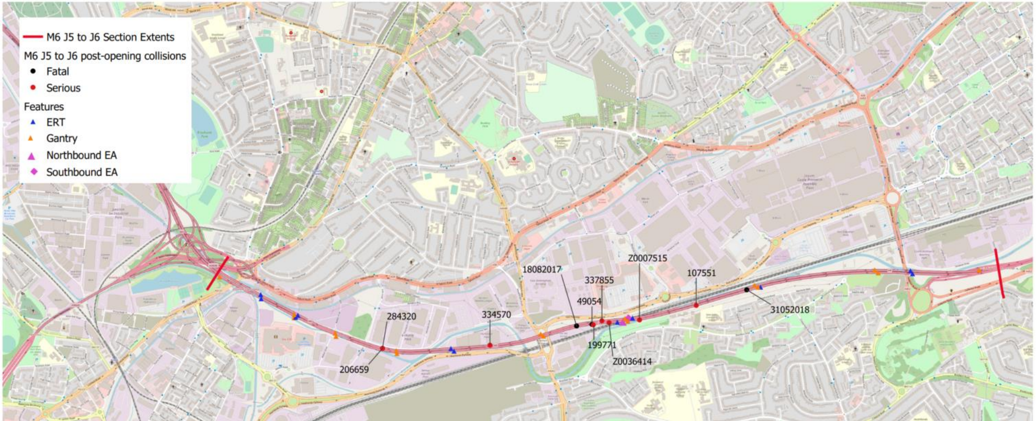
Figure 5.1 Location of fatal and serious collisions (including emergency telephones and signal gantry locations)
