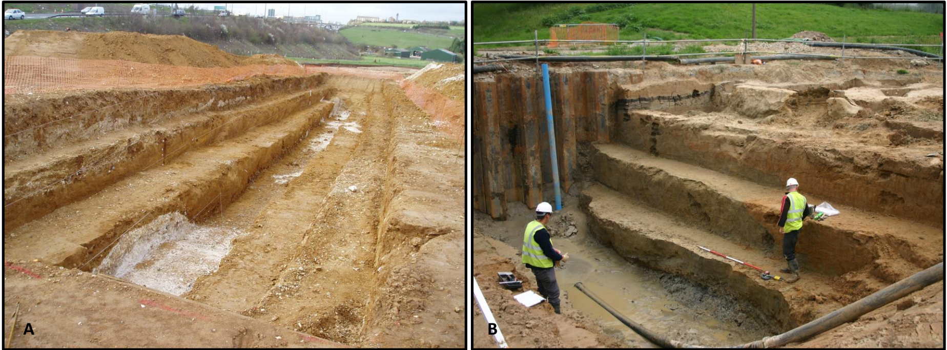
Figure 18. Slopewash deposits: A) slopewash sands and gravels probably deposited under periglacial conditions at Dartford (M25/A2 junction, Link C, TP 8800); B) slopewash sands (derived from Thanet Sand) overlying cold stage fluvial gravels at Northfleet Waste-water Treatment Works.
