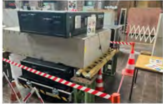
GSCAN muon detectors in BAM lab
