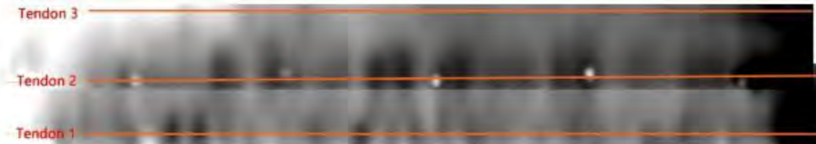
figure 6-3: The magnetic picture from figure 6-1 with marking of the position of tendons 1 to 3
