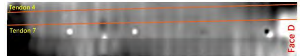
figure 6-5: The magnet picture of face E with the tendons 4 and 7
