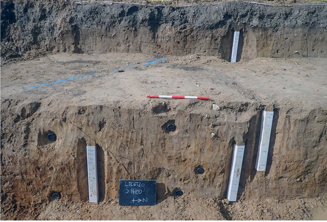
Plate 17: Geotechnical Section 14100 showing location of samples
