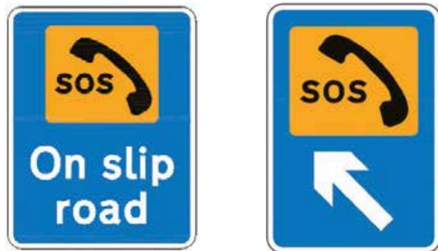
Figure 9 Approach signs indicating the presence of an emergency roadside telephone adjacent to hard shoulder on an exit slip road
