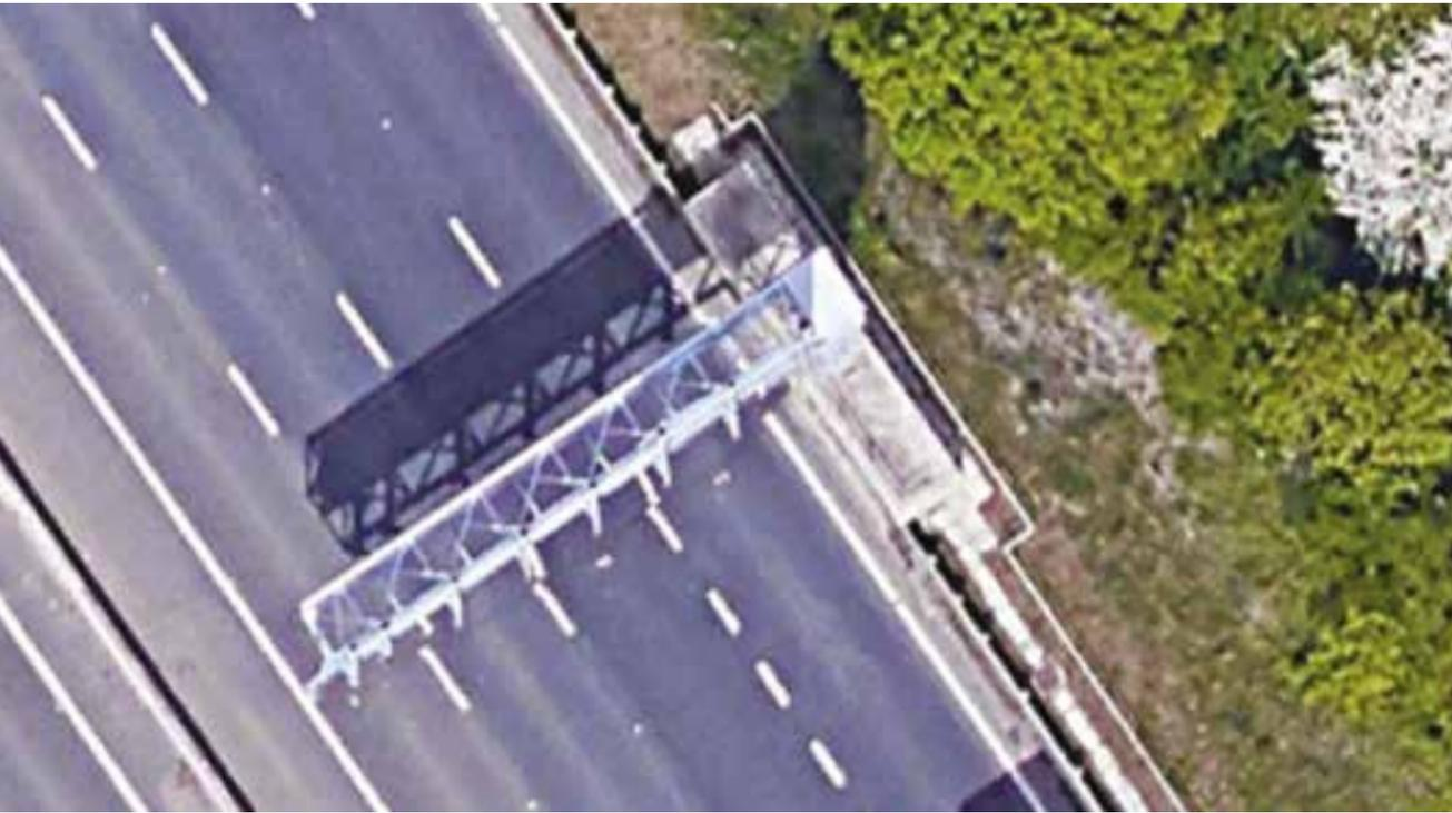
Figure 5 Change in lane markings between lane 1 and 2 at the 1/2 mile marker to the junction © Google
