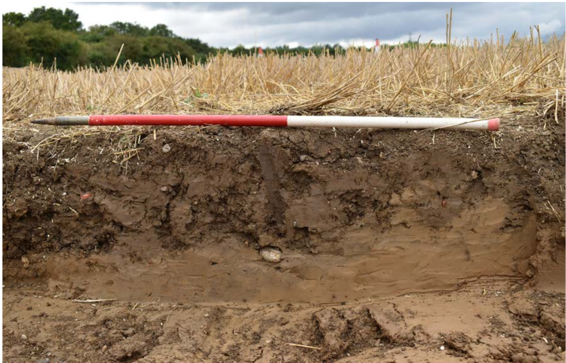
Plate 31: Trench 104, Section 10400, showing shallow Head deposits over London Clay on the southern slopes of Land Parcel 126
