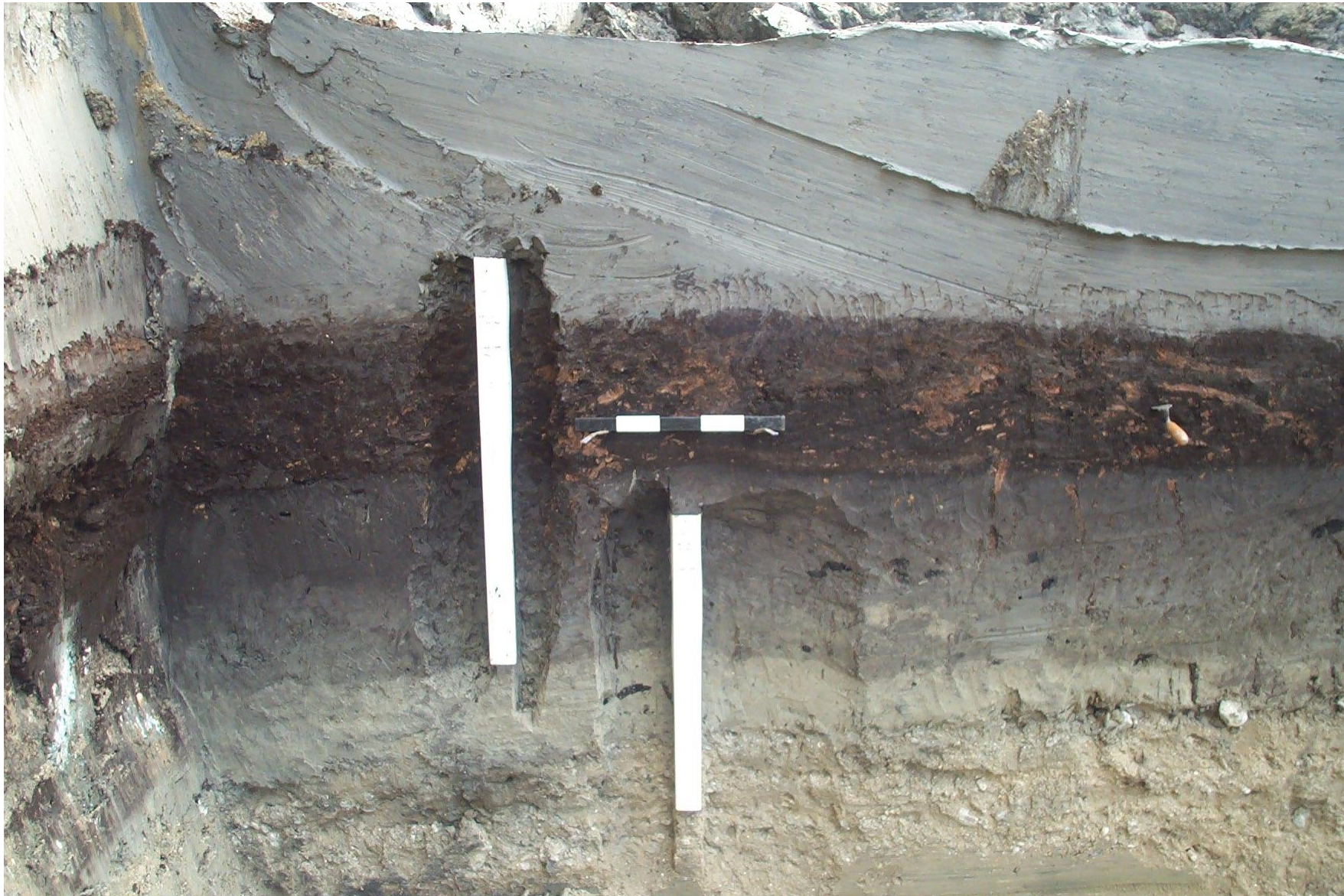
Figure 22. Basal peat overlying weathered surface on top of Late Pleistocene fluvial gravels at the Thames River Crossing (south portal) site on High Speed 1 line.
