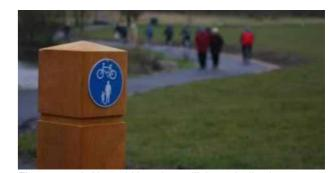
Figure 90. A Shared Use sign utilising a bollard
