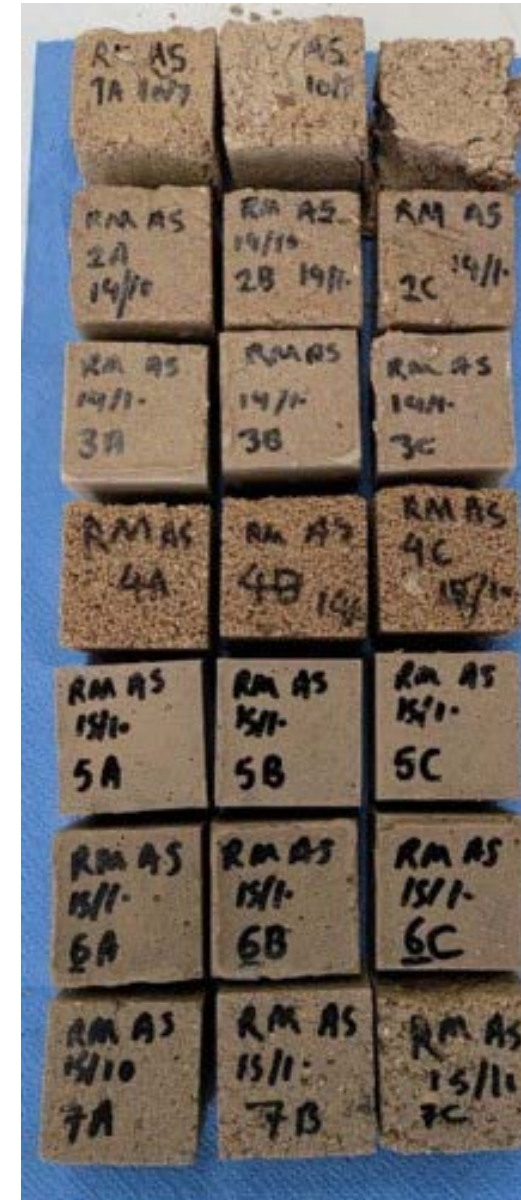
Geopolymer mortar specimens containing waste calcined clay or pure clay
