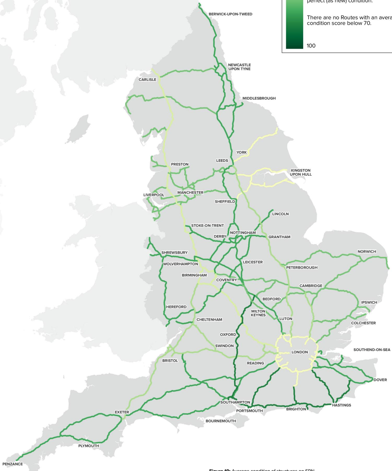
**Figure 19:** Average condition of structures on SRN
